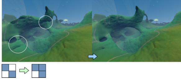
Fig.13. Smoothing errors: Applying a simple filter operation on the volume data can avoid most problems (Marked by white circles). The filter seeks the left pattern shown below and replaces it by the right one.
